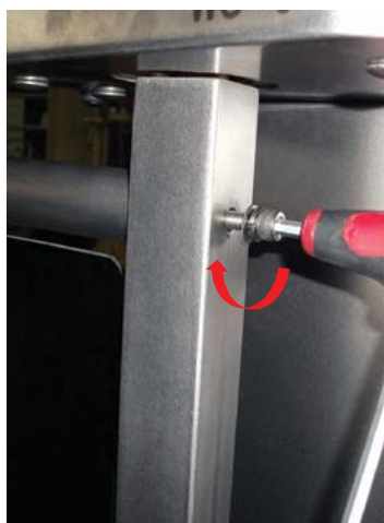
2. Tighten top fixing screw
