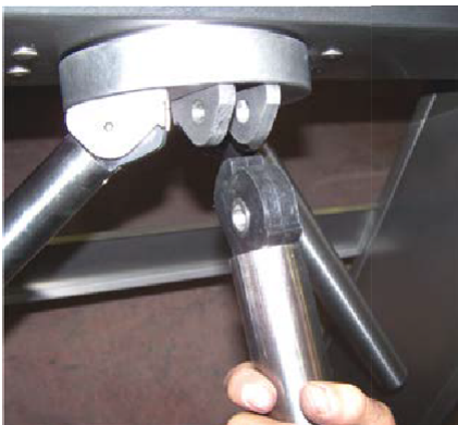
Seat the arm on the rotor
