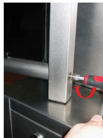
3. Tighten bottom fixing screw
